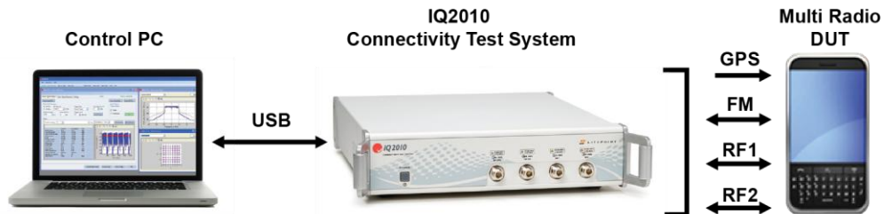
Figure 2: IQ201X Test System—Testing Connectivity Functions of a Mobile Device
