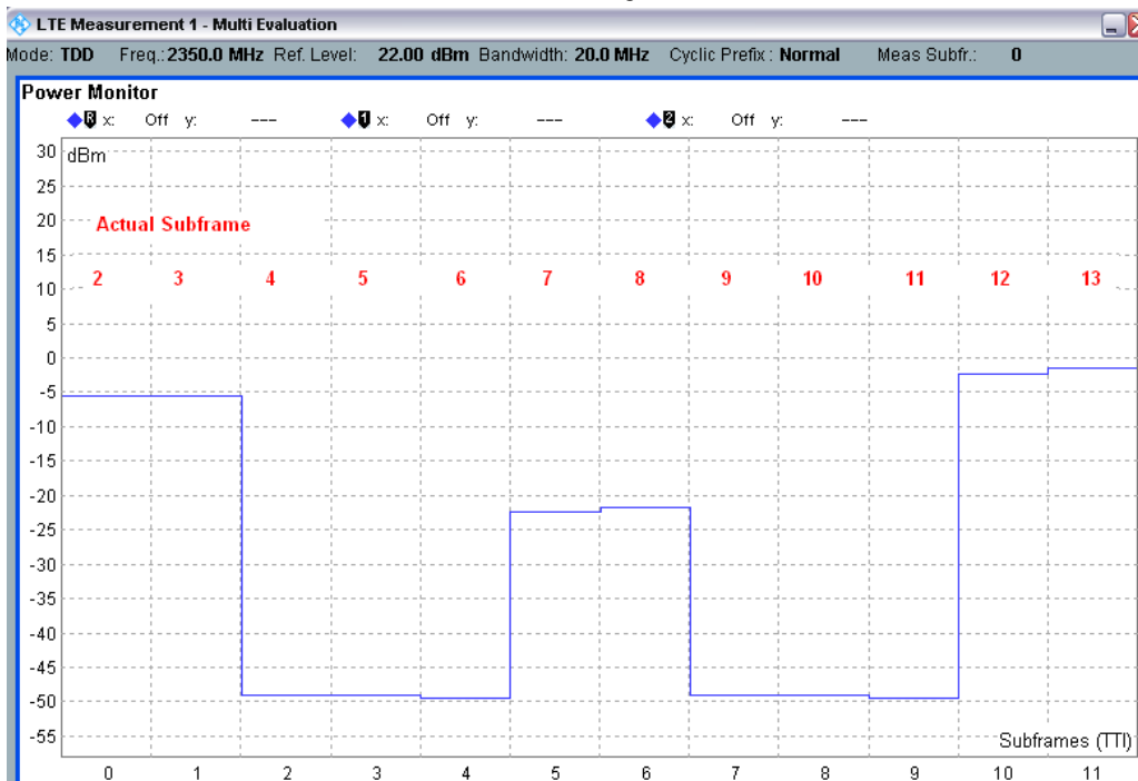
b) Measurement Trace for the frame with RB change for TDD
